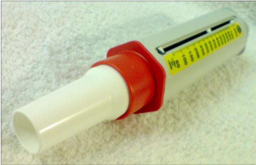
This is a peak flow meter, which measures air pushed out from the lungs.
